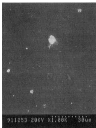
Figure 2. SEM image of polyimide LB film deposited HOPG substrate.
